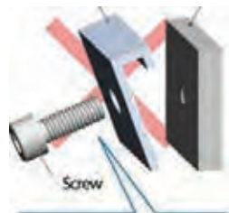
Screws fall out when the cover is removed.
